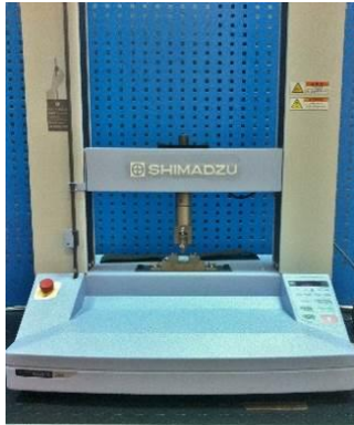
Fig. 6. A universal flexural test device (İzmir Katip Celebi University, Mechanical Engineering Laboratories)
