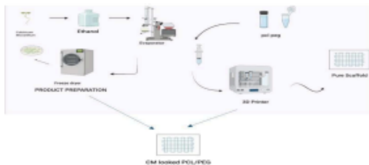
Figure 1. Schematic overview of the study workflow. The figure illustrates: (i) preparation and lyophilization of Colchicum extract; (ii) formulation of PCL/PEG composite solutions; (iii) 3D scaffold fabrication by extrusion-based 3D printing.
